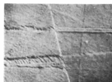
Fig. 18. (a) and (b). Abrasion grooves crossing a grain-boundary in polycrystalline Be.
