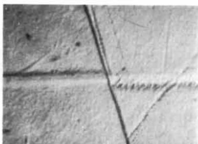
Fig. 18. (a) and (b). Abrasion grooves crossing a grain-boundary in polycrystalline Be.
