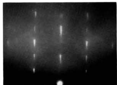
Fig. 8. Electropolished Be ( 0001 ) face; beam [100] .
